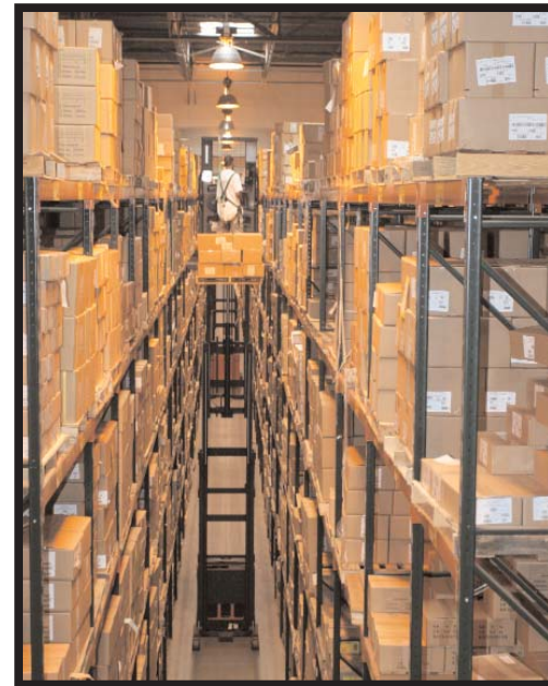
Tethered by a safety strap, a VHPS employee uses a forklift to gingerly lower a pallet load of books from three stories up at the 450,000 square foot book distribution and warehousing facility. Note the wire guidance system in the floor that keeps the fork lift centered in the aisle. Photo by Phil Audibert
